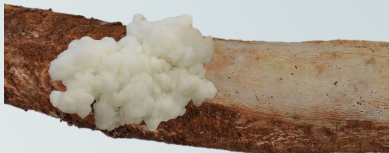
Fig. 3: Hydro-alcoholic solutions and anionic surfactants, applied with a poultice.
