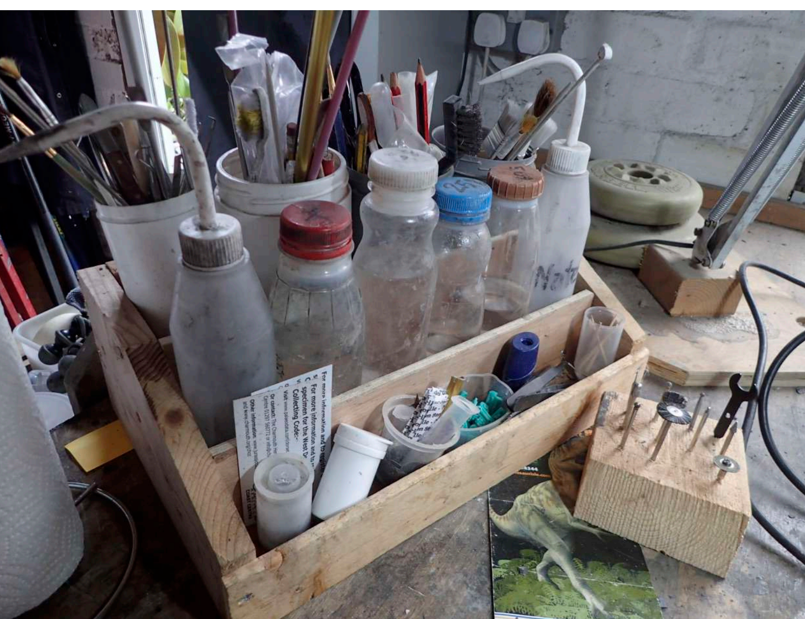
Adhesives and solvents and all sorts of different tools and applicators. I have this as a standard set-up so that I can reach for the correct bottle without looking. Left to right: acetone spray, acetone in bottle, 50% paraloid, 25% paraloid, 10% paraloid, water spray. For weaker paraloid solutions I add acetone to a small pot of 10% mix.
