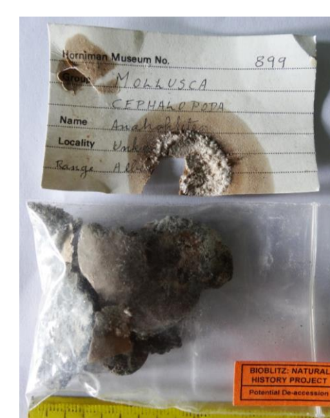
Here pyrite decay has damaged both the specimen and its label. © Horniman Museum and Gardens.
