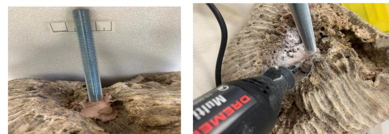
Process of removing the metal stand with Dremel
