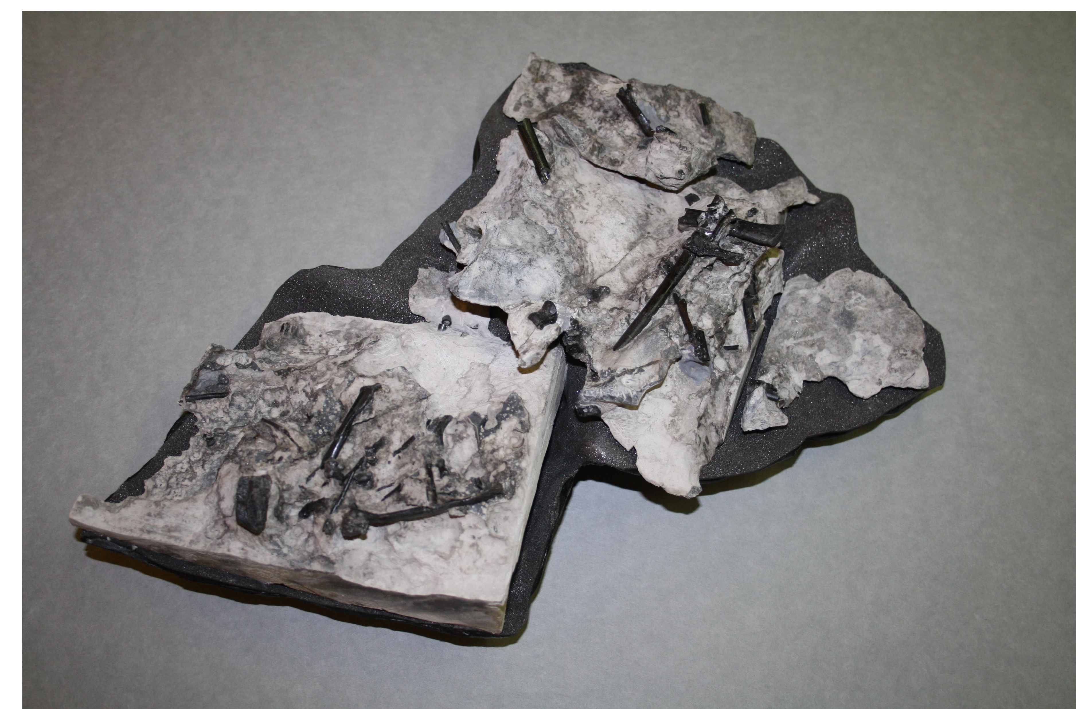
The blocks are now stored in an Epopast 400 mount, covered with Plastazote foam.
