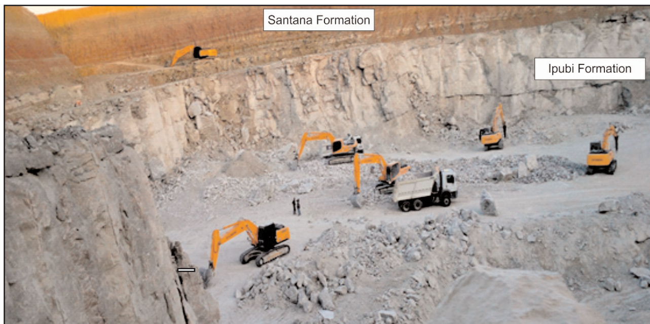
Figure 3. In this quarry near Ipubi, Ceará State, Brazil, the Santana Formation Fossil Lagerstätte with its fossil-bearing nodules is removed to expose the valuable gypsum beds of the Ipubi Formation. The fossiliferous nodules are simply thrown on to the spoil dumps. No one makes any effort to collect them.
