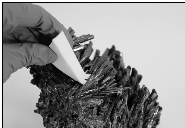
Figure 2. The finer topography of this stibnite is more effectively cleaned using a small scarified piece of cosmetic sponge. Natural History Museum specimen; Lu Allington-Jones photo.
