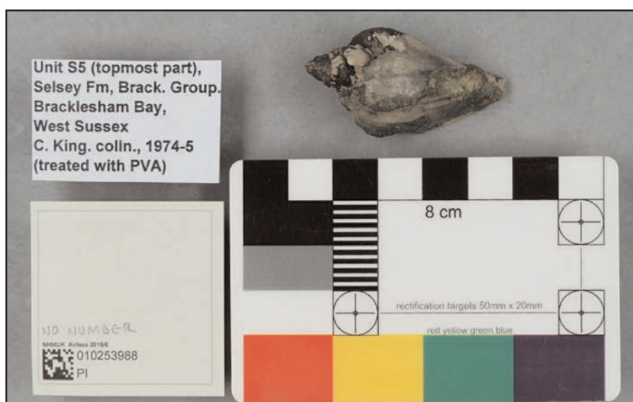
Figure 6. Gastropod (NHMUK PI TG 27057) with label describing treatment (date unknown): "treated with PVA". Specimen shows signs of hardened decay products on the surface.
