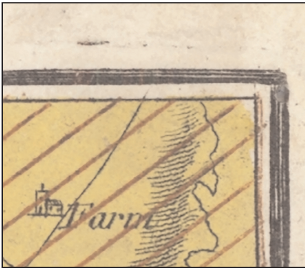
Figure 3. Detail of the upper right corner of the Bath map showing the plate mark where the edge of the copper plate pressed into the paper during printing (Conybeare and De la Beche 1823). Reproduced by permission of the British Geological Survey CP 18/044.
