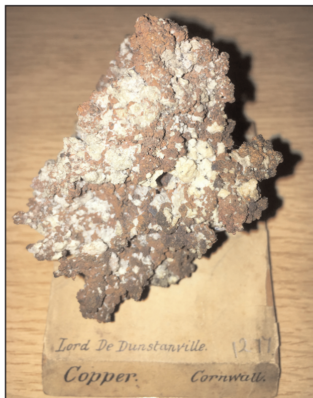
Figure 12. Native copper. Specimen 7 cm across. A dense aggregate of hackly native copper intergrown with milky quartz.
