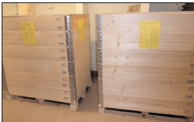
Figure 3: Wooden crates formed using collars placed around drawers and shelves on pallets.
