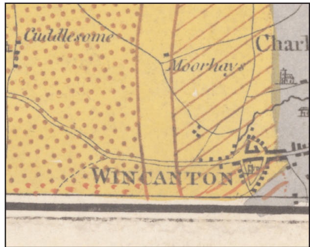
Figure 5. Detail of the bottom edge of the Bath map showing hand-painted dots and lines filling in the registration gap caused by mis-alignment of the red patterns printed from the second plate with the black border on the base map plate (Conybeare and De la Beche 1823). Reproduced by permission of the British Geological Survey CP 18/044.
