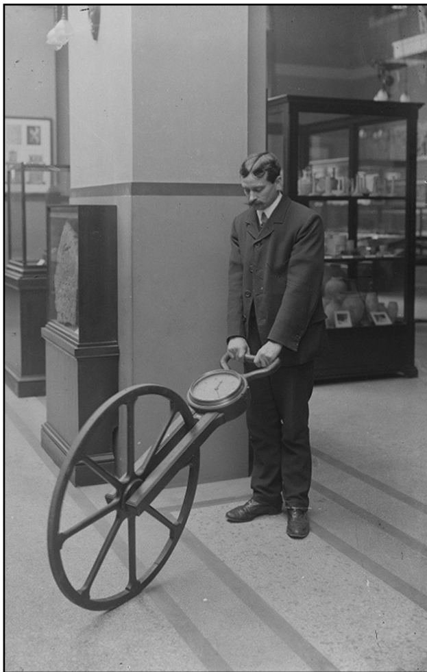
Figure 6. 1939 image of a wooden road measuring wheel or 'waywiser' used by George Ashmead, cartographer, Bristol c. 1825-1835 for surveying Bristol streets. BRSMG J2760. © Bristol Culture.
