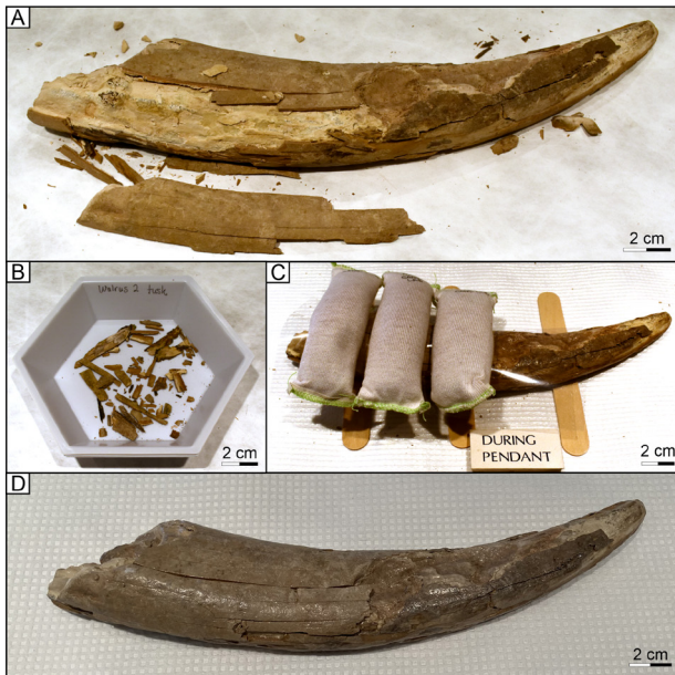
Figure 7. Semi-fossil walrus tusk (NBMG 21606) showing spalling A) during slow, controlled, drying following desalination, including small fragments, B) the same specimen during consolidation and reconstruction, C) with weights and a mylar shield in place and D) the fully consolidated and reconstructed tusk.
