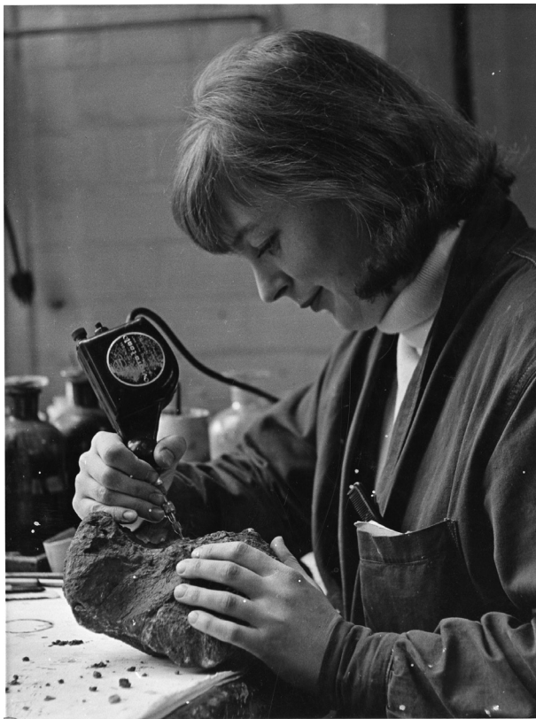
Figure 2. Judy Goodall preparing a fossil with a vibro-tool, 1969. Natural History Museum Archives, TCC-ARC-1702a.
