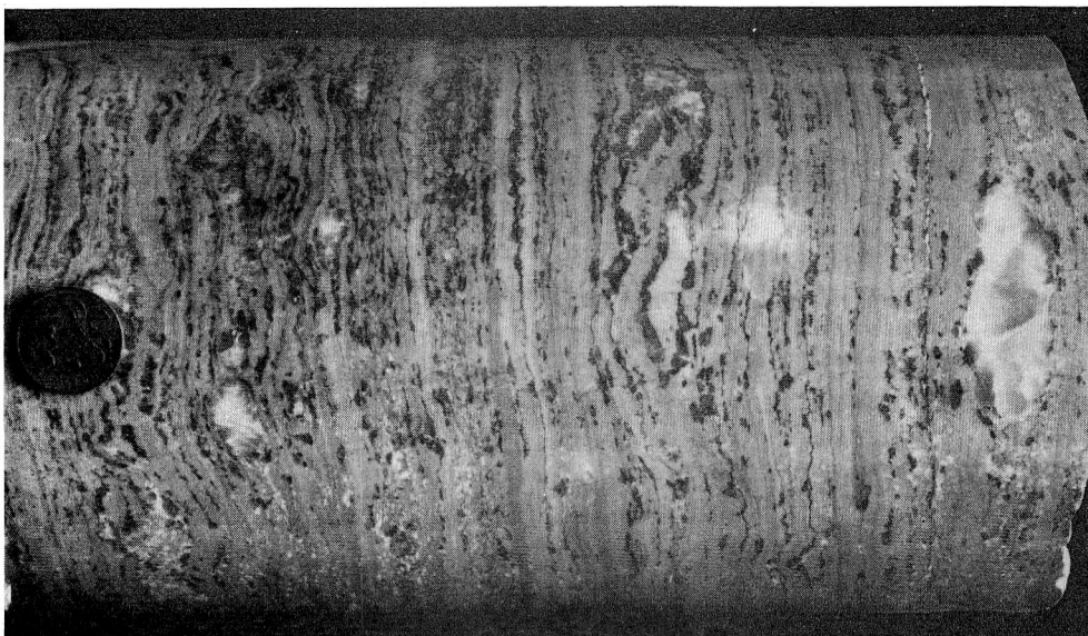
Fig. 3. Part of a polished core (35cm. x 16.8cm diameter) showing algal-laminated (stromatolitic) dolomite with displacive nodules of anhydrite and gypsum. Permian Hartlepool Anhydrite Formation from an N.C.B. offshore borehole, north-east coast.
