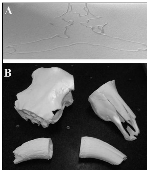
*Figure 5. One of the layers after sintering with the CO<sub>2</sub> laser (A) and the four pieces of the urus cranium replica (B).*
