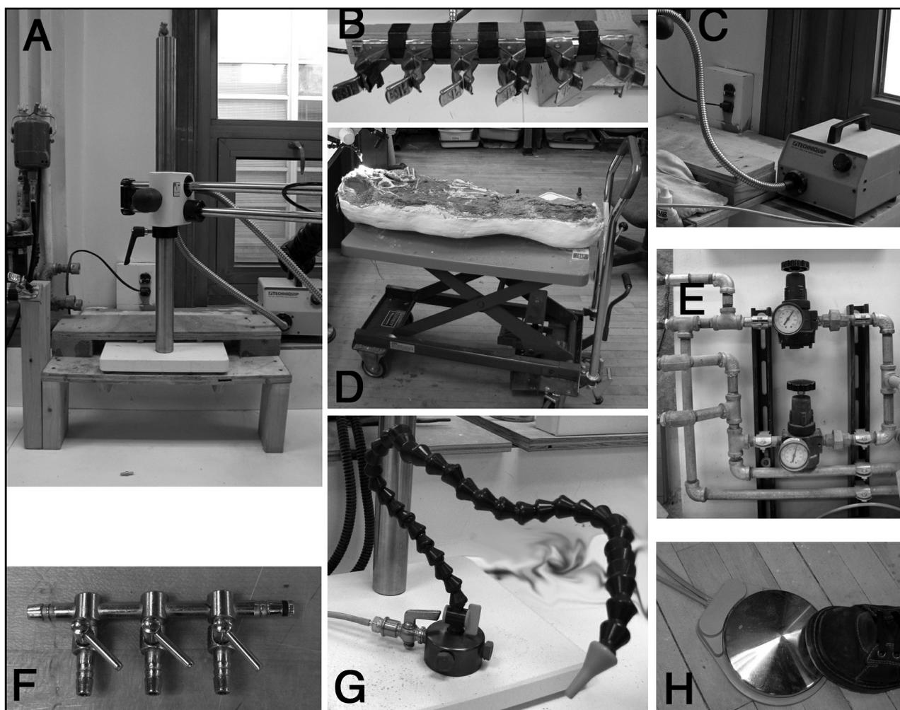
**Figure 1.** (a) Microscope platform, (b) spring clips, (c) light box, (d) hydraulic lift table, (e) compressed air gauges, (f) air supply gang valve, (g) modular tubing, (h) foot pedal.
