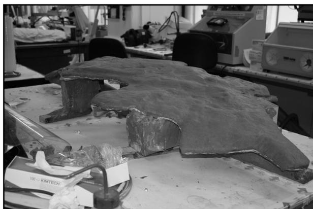
**Figure 10. Epopast support on specimen.**
