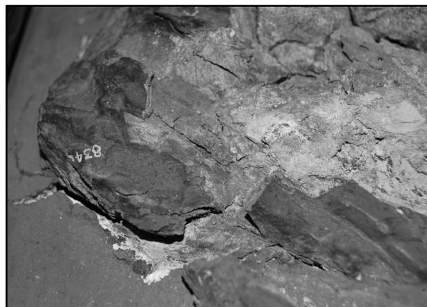
**Figure 2 White sulphuric deposits from pyrite decay.**
