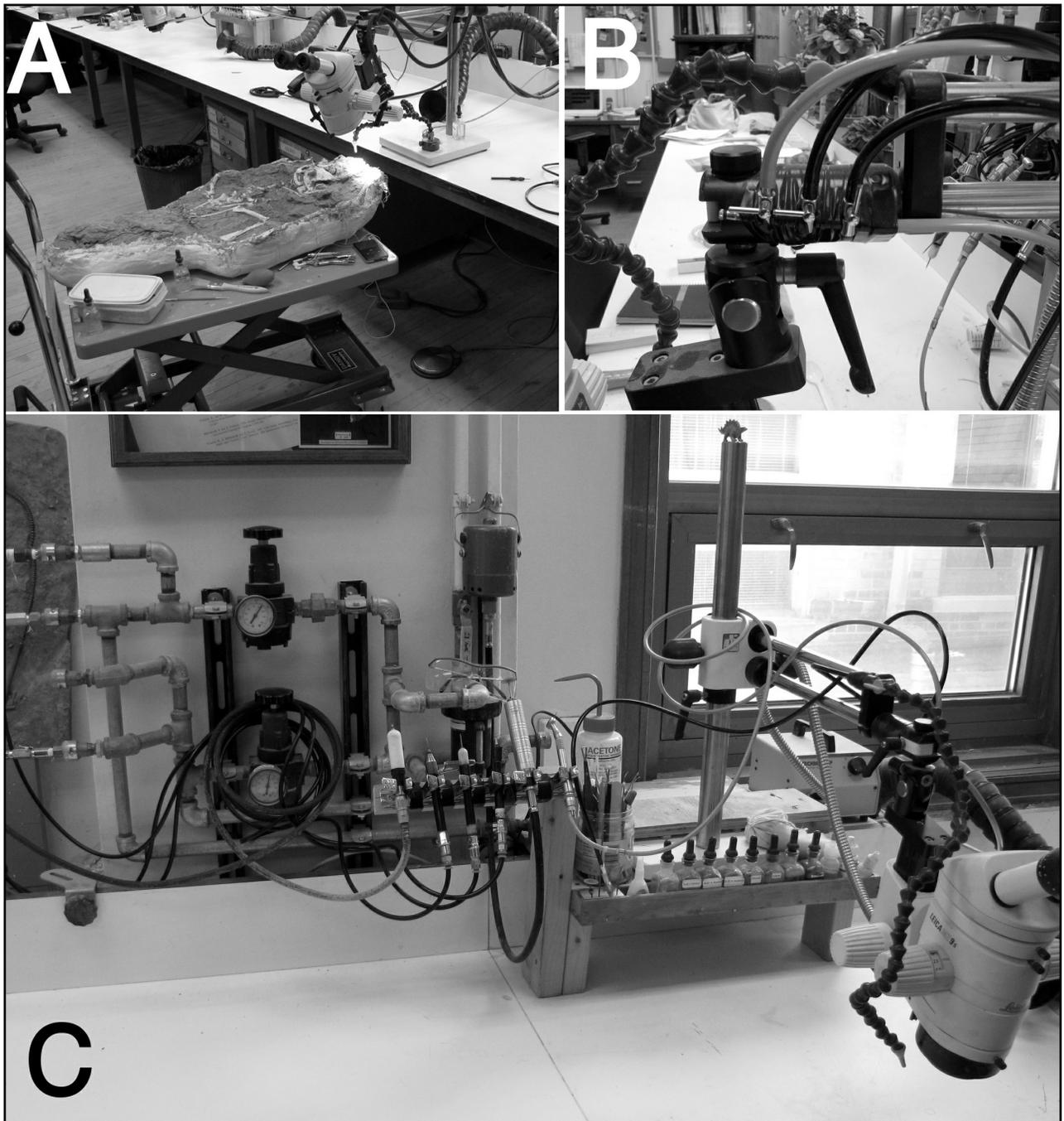
**Figure 2:** (a) Hydraulic lift table with microscope, (b) Gang valve mounted on microscope arm, (c) Workstation setup.
