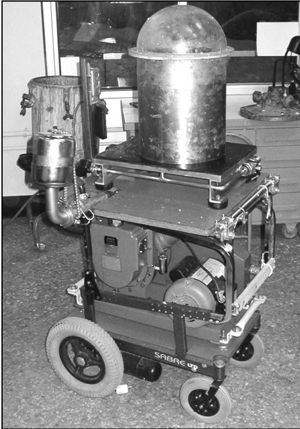
*Figure 3. Because FossiLab did not contain them, P. Reser's fast-cycling portable vacuum chamber and pump, which is more efficient than those found in most labs, was brought in for the training. A pressure pot, also used in the resin casting, is visible in the left background.*
