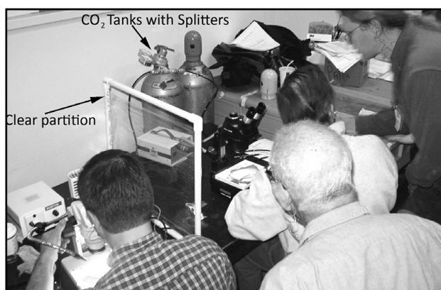
**Figure 2.** Training workstations with binocular dissecting microscopes and directional fiber-optic lights, air scribes, portable partitions made of PVC and plastic wrap, and CO<sub>2</sub> tanks with splitters to run two tools off of each tank.
